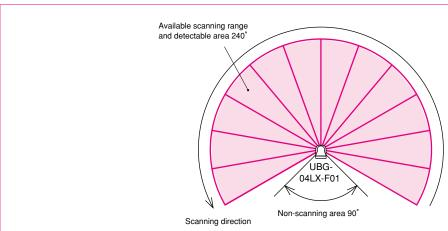
note) The above figure shows the detectable area for white Kent sheet (80mm×80mm) and max. distance is 4m. Detection distance may vary with size and object.
