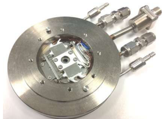
The window and mirror of 13mm diameter are available to set on the sample port
