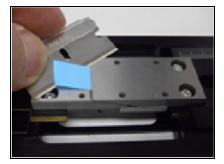
Standard MicroVice Clamps 90° Cutting Angle
