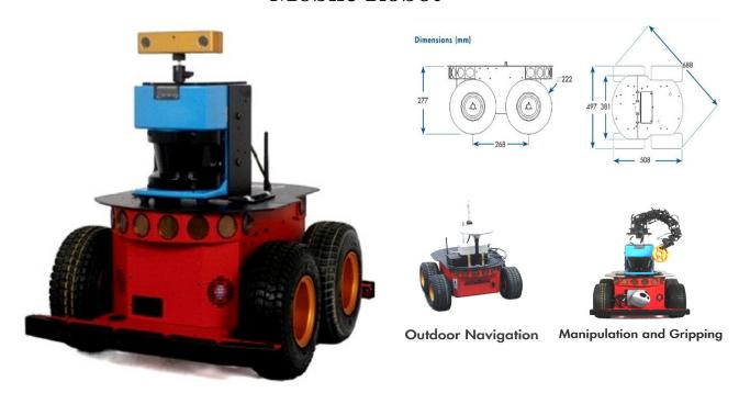
The Mobile Robot platform is the basic mobile setup required to perform mobility experiments, navigation, mapping and other behaviors. It is a combination of various physical components (hardware) and computational (software) components.
